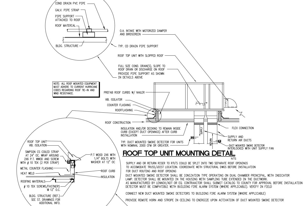
TYPICAL ROOF TOP UNITS MOUNTING DETAILS
